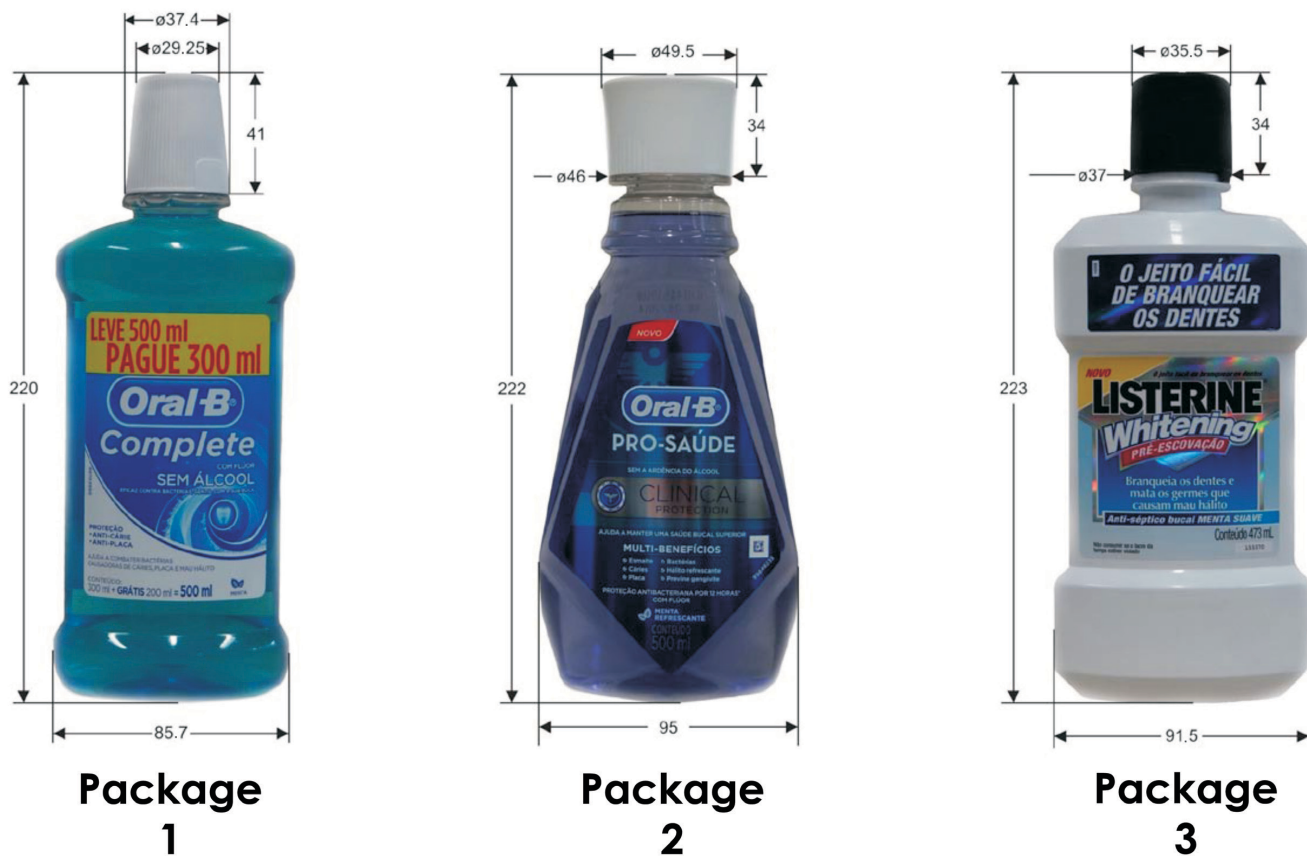
Figure 1. Selected packages (the dimensions are in millimeters).
